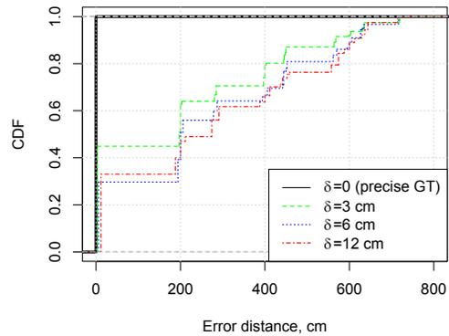
Fig. 7. Two-dataset positioning performance with different GT errors.
