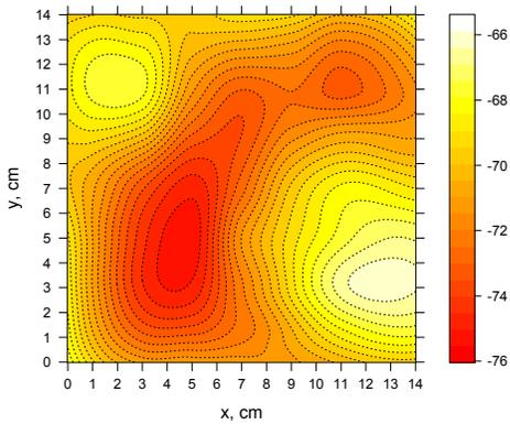
Fig. 1. Small-scale fading of Wi-Fi signals. Empirical measurements show 10 dB RSS variations in a  $14 \times 14$  cm area sampled with 1 cm resolution.
