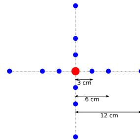
Fig. 5. Layout of a test location: central test point (red) surrounded with auxiliary test points (blue).
