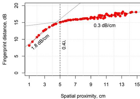
Fig. 3. Experimentally measured similarity between Wi-Fi RSS fingerprints in nearby points (indoor measurements).
