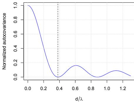
Fig. 2. Theoretical covariance of signal amplitudes received in two points distance  $d$  apart, in a multipath environment [27, Eq. 16].
